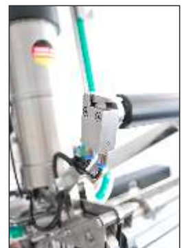
Messer- und Schlaufenauslösung in VA Knife and loop release made in stainless steel
